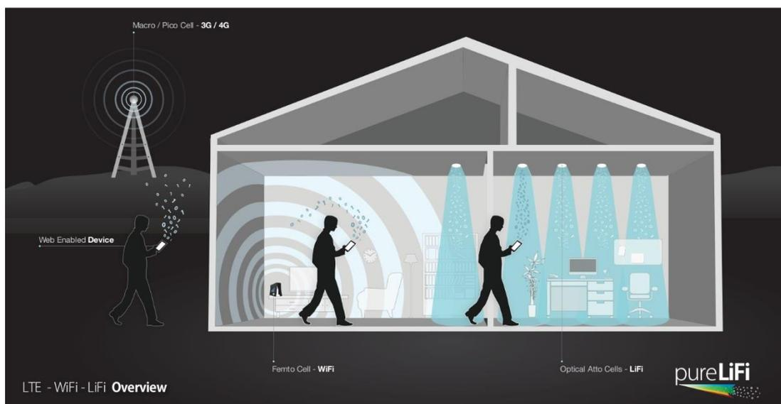
*LiFi works in complement with existing and emerging wireless systems (source: pureLiFi).*
