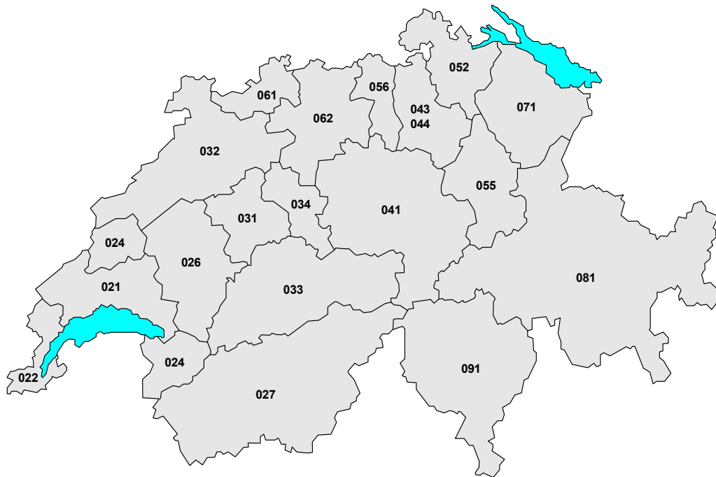
Figure 1: National destination codes for fixed network services in the E.164 numbering plan
